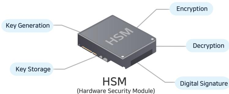
The tried-and-true way to safely store keys is to use a hardware appliance called a Hardware Security Module (HSM). An HSM safeguards cryptographic keys, and it supports the lifecycle of key management and various cryptographic operations such as encryption, digital signature, and more.
