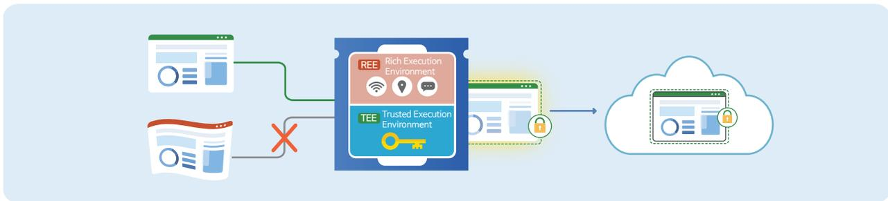
TEE creates a secure area inside the main processor, isolated from the Regular Execution Environment (REE). In the trusted area, only authorized programs can run and access sensitive information.
